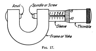
thousandths of an inch. The micrometer in Fig. 17 reads as follows:
