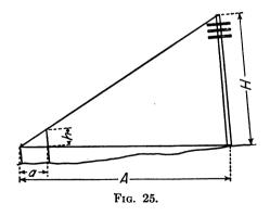
"h" may be found. The distances from the top of the short pole to the foot of the telegraph pole, that is distance "A" and also distance "a" (from the top of the
