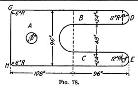
25. Figure 78 shows the top sheet of a tank made of ¾-in-steel plate. Find its area by dividing it into rectangles as shown by the dotted lines.
