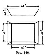
13. Find the contents in cu. in. of the drip pan shown in Fig. 146. How many gallons will the pan hold?
