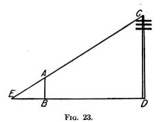
The distance BE is measured and knowing distances DBE and BE, distance CD can be easily calculated.
