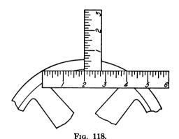
segment thus formed. The diameter then equals the square of one-half the length of chord plus the square of the height of segment all divided by the height of segment. To apply this rule in finding the diameter of the broken pulley shown in Fig. 118, the length of the chord measures 4 in. and the height of segment  $9_{16}$  in.
