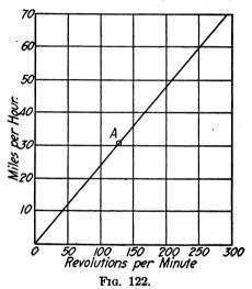
per hr., which is about as high a speed as it is safe for a locomotive to run. The corresponding highest number of revolutions per min. is approximately 295. In order therefore to get these values on the sheet we use the scales as shown. The small circles show the location of the points plotted from the figures in the table. These points lie along a straight line from which we can find the speed for any given number of revolutions per min.,
