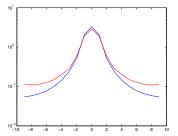
(Right) Actual function (blue) vs. the function reconstructed from the FFT coefficients (red)
